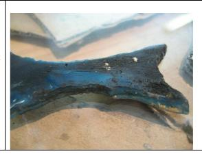
To get rid of the soot, the pieces of glass are soaked for 1 hour in a solution of 75 % warm water and 25 % of "Simple Green", an organic detergent, very effective in removing the dirt.
