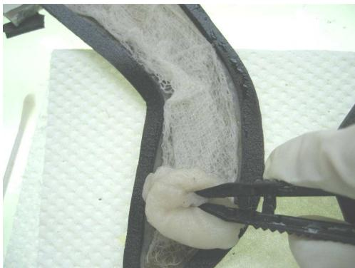
After half an hour, the pieces of gauze containing the solution are removed and the pieces of glass
