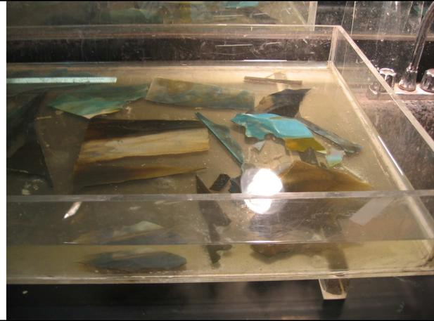
The pieces are being soaked in a solution of 10% lye and 90% of warm water for half an hour.
