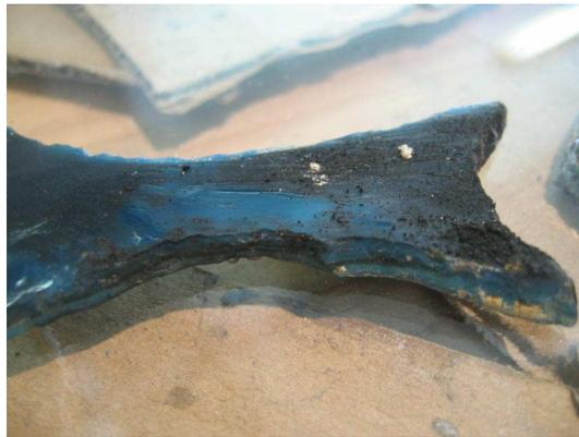
To get rid of the soot, the pieces of glass are soaked for 1 hour in a solution of 75 % warm water and 25 % of “Simple Green”, an organic detergent, very effective in removing the dirt.
