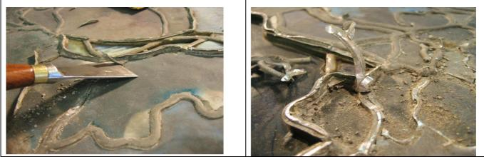
The upper wing of the lead is peeled away using a sharp knife, leaving the heart and the lower part of the lead.
